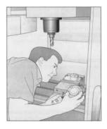
Don not get caught up in your work! All milling machines contain hazards from rotating parts, belts and pulleys, high voltage electricity, noise, and compressed air. When using CNC machines and their components, basic safety precautions must always be followed to reduce the risk of personal injury and mechanical damage.
