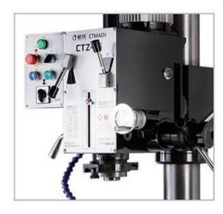
The spindle box can be raised and lowered and can also rotate 360° around the column. The middle worktable can also swing ±90° and tilt back and forth 45°.
